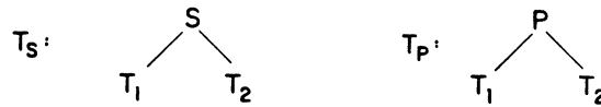
FIG. 4. Rules to construct T_S and T_P (the binary decomposition trees of G_S and G_P in Definition 1) from T_1 and T_2 (the binary decomposition trees of G_1 and G_2 ).
